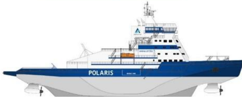
IB Polaris (2016) World's first LNG powered icebreaker, in-built oil recovery system PC4
